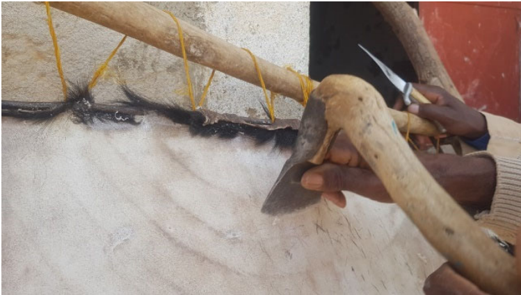
Fig. 9. Frame for stretching skins (with inserted iron rods), adze-like instrument used for scraping the hair-side (photo-credit: Hagos Gebremariam)
