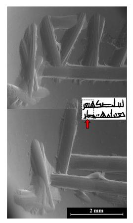
Figure 6. ESEM-EDS general observation of the crystal gem, showing two lines of engraved letters (at the left side of the object, arrow).
