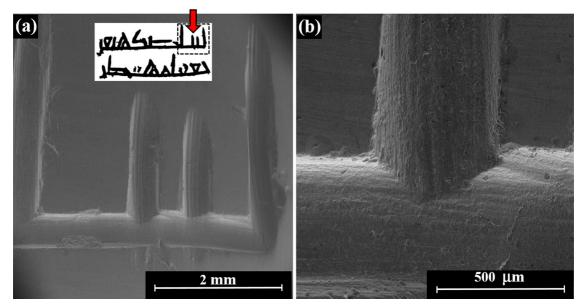
Figure 7. ESEM-EDS examination of the crystal gem: (a) general view of one of the engraved letters (right upper side of the object, arrow); and (b) ESEM higher magnification showing the roughness of the examined engraved letter.
