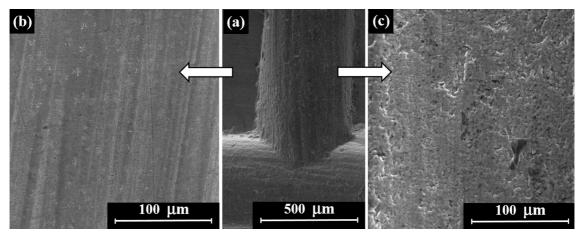
Figure 8. ESEM-EDS examination of the crystal gem: (a) general view of one of the engraved lines (shown in Figure 7); (b) the polished surface of the crystal gem (outside the letter, left arrow) produced by abrasive particles; and (c) the rough surface inside the engraved letter.
